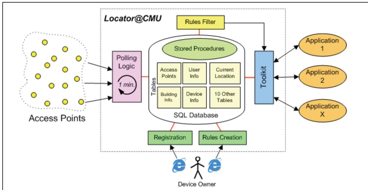
**Figure 1: *Locator@CMU System Diagram***, all campus access points are polled every minute, information is stored in the *Locator@CMU* system (dotted line). Wearable and context-aware applications utilize the associated toolkit to access data.
