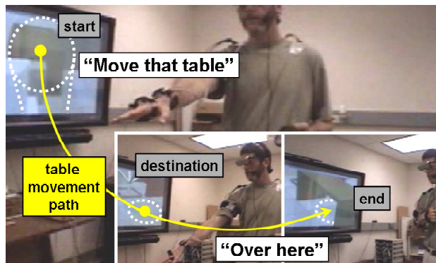
Figure 1: A 4-part multimodal command (speech/point + speech/point) to move a virtual table. The plasma screen shows what the user sees in his HMD. The white-dotted areas (added here) show pointing targets. Turn segmentation is critical to correct multimodal recognition.
