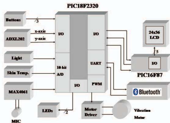
Figure 2. Hardware architecture
