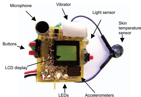
Figure 3. eWatch controller board
